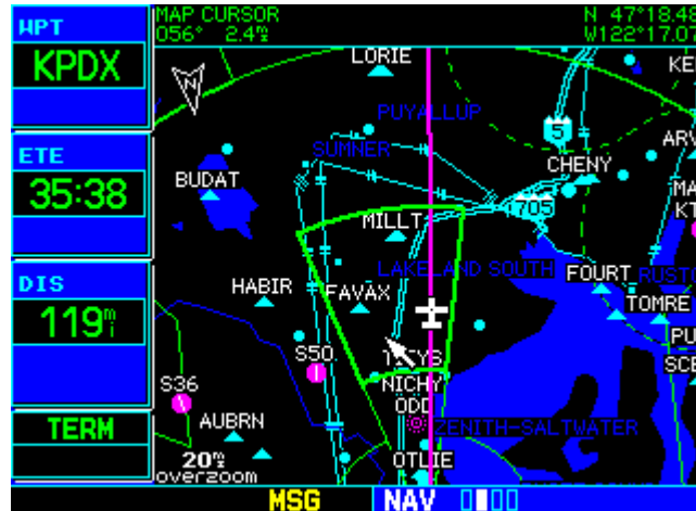
Once activated, the flight plan can be displayed on the map page.
