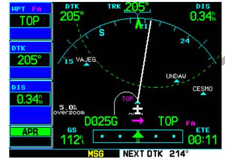
STEP 9: As you approach the FAF, a "NEXT DTK 214°" waypoint alert will appear in the lower right corner of the screen.
